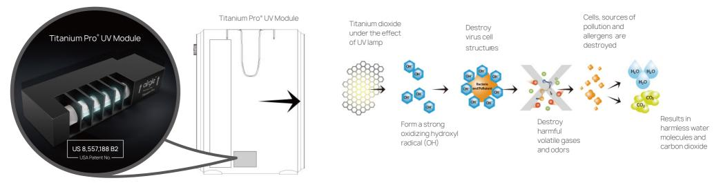
1) The Titanium Pro<sup>®</sup> module creates hydroxyl radicals by exposing titanium oxide (TiO<sub>2</sub>) to ultraviolet light. Hydroxyl radicals are naturally occurring molecules in the atmosphere. In fact, they are often referred to as the "detergent of the troposphere" because hydroxyl radicals destroy many airborne pollutants by breaking apart the molecules of the pollutant.
